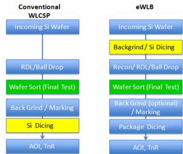
Figure 4. Process flow of WLCSP and eWLB
